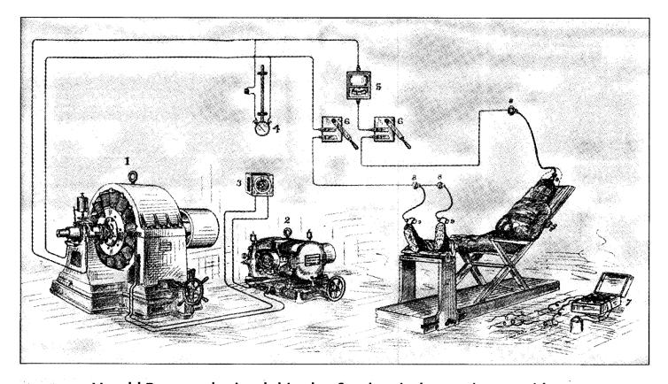
Harold Brown submitted this plan for electrical execution as evidence during the hearings phase of Kemmler's appeal. On the generator he added a label reading "Westinghouse Electric, Pittsburgh."
